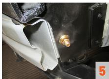
Using the two rear holes as a guide, drill 13/32" holes in the vehicle frame. Position the driver-side tow bar base plate mounting bracket (#2) and fishwire two 3/8" x 2" carriage bolts (#8) with square hole spacers (#6) and secure them with 3/8" flange nuts (#9).
